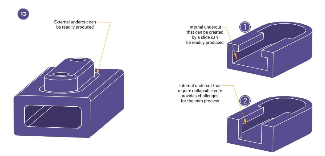
Generally though, MIM components are small and collapsible cores are often impractical and sometimes impossible to produce. Collapsible cores also provide challenges in maintenance to minimize flash. Please seek advice from our engineers when considering such features.
