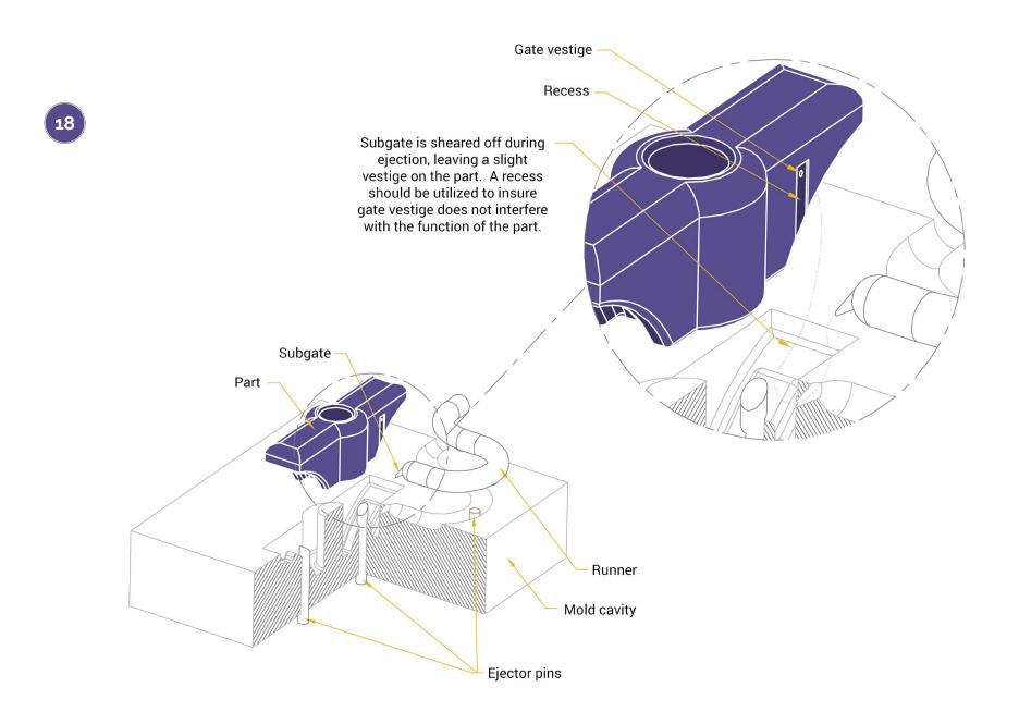
Fig. 19 illustrates a submarine or sub-gate to a removable post. This gating approach has the following characteristics:
