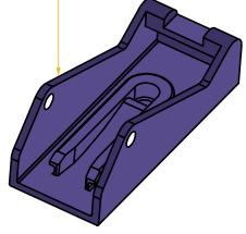
CNC Machined part is welded onto the stamping
